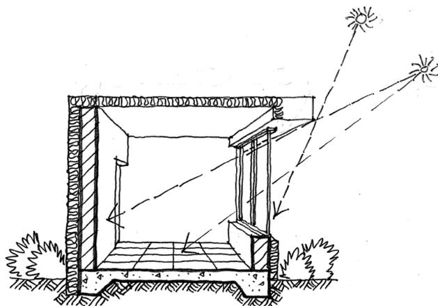
*Properly accounting for this change of Sun angle when orienting and designing a house can significantly reduce the need for heating and cooling.*
