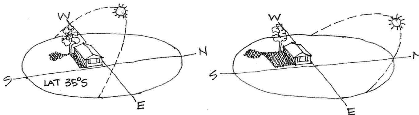
Figure 2 – correct orientation maximises exposure to sunlight in winter, minimises exposure to sunlight in summer
